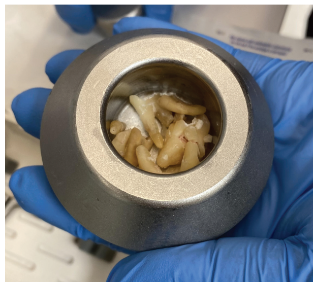
Figure 5. Trimmed and dried teeth inside surgical mortar before being placed in one of the mills.
